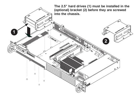
Figure 6-4. Installing 2.5" Hard Drives
